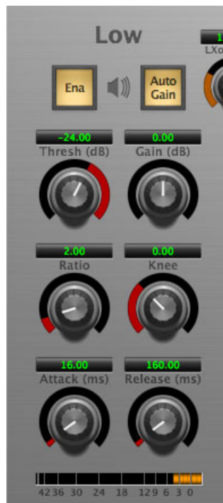
Figure 5.4: Compressor (Low Frequency Shown)
